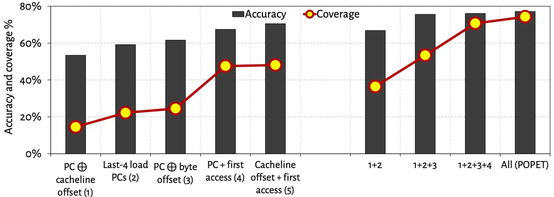
**Combination of features** provides both **higher accuracy and higher coverage** than any individual feature
