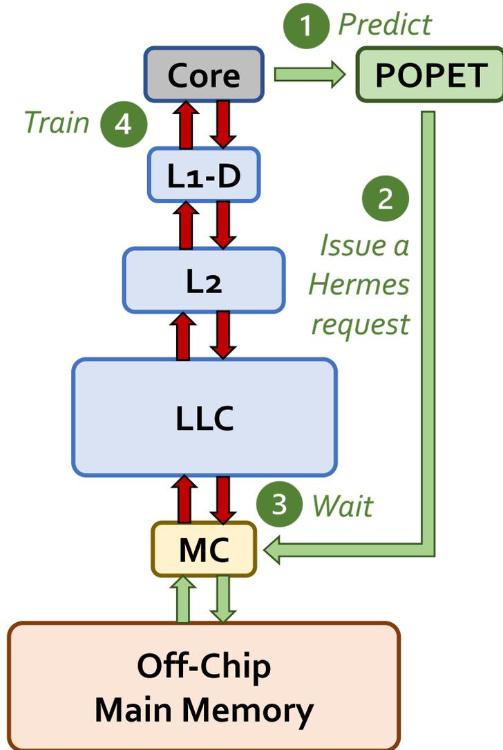
Perceptron-based off-chip load predictor
