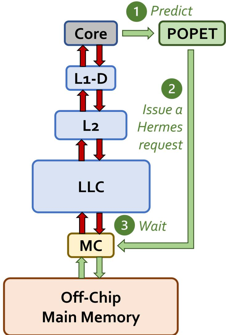
Perceptron-based off-chip load predictor
