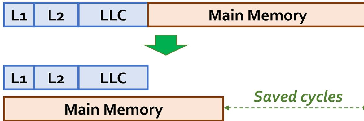
**40%** of the **stalls** can be eliminated by **removing on-chip cache access latency from critical path**
