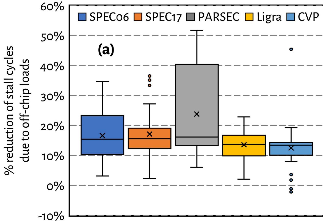
Hermes reduces off-chip load induced stall cycles on average by **16.2%** (up-to **51.8%**)
