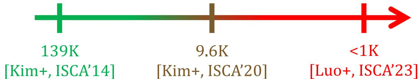
Mitigation mechanisms against RowHammer attacks **induce higher overheads** as **RowHammer worsens**
