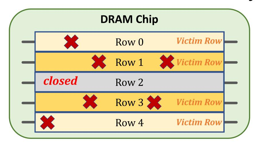
Repeatedly **opening** (activating) and **closing** (precharging) a DRAM row causes **RowHammer bit flips** in nearby cells
