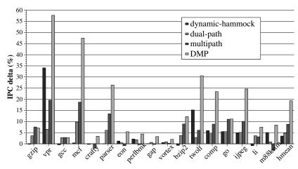
Figure 6. Performance improvement provided by DMP vs. dynamic-hammock-predication, dual-path, and multipath execution
