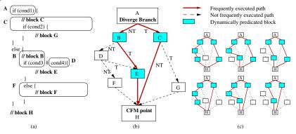
Figure 1. Control-flow graph (CFG) example: (a) source code (b) CFG (c) possible paths (hammocks) that can be predicated by DMP
