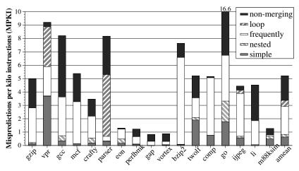
Figure 5. Distribution of mispredicted branches based on CFG type
