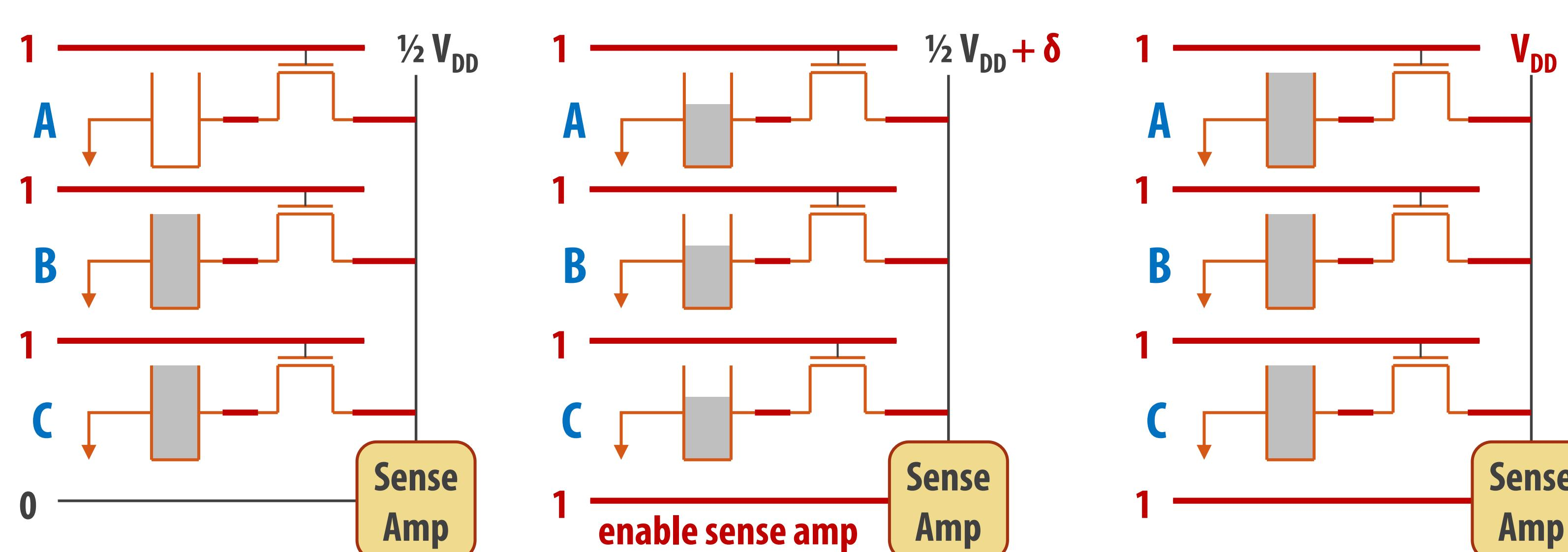
$$\text{Output} = AB + BC + CA \\ C(A \text{ or } B) + \sim C(A \text{ and } B)$$
