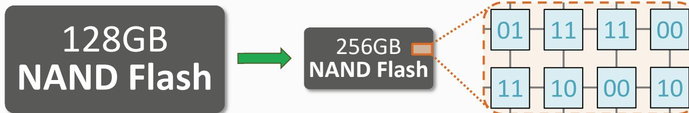
NAND flash scaling: **shrink size** of each flash cell, **store *two bits*** per cell
