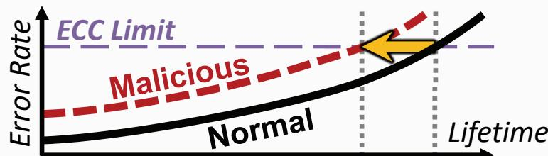
Vulnerabilities can be **exploited** to corrupt data and **reduce flash lifetime**
