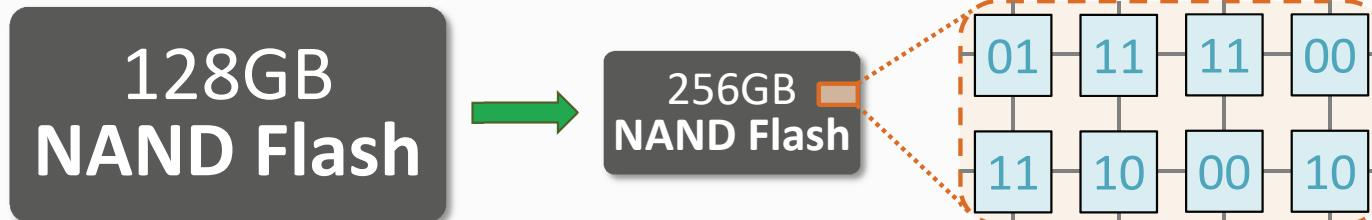
NAND flash scaling: **shrink size** of each flash cell, **store *two bits*** per cell
