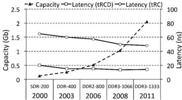
Fig. 3 DRAM Capacity & Latency Over Time. Reproduced from [106].
