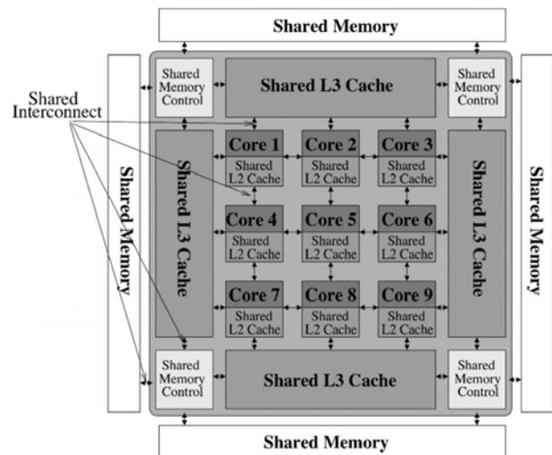
Fig. 8 A typical multicore system. Reproduced from [130].
