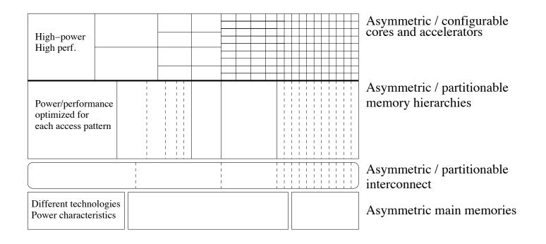
Design each hardware resource with asymmetric, (re-)configurable, partitionable components
