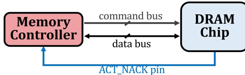
Leveraging the ability to *reject an ACT*, a **maintenance operation** can be implemented **completely within a DRAM chip**
