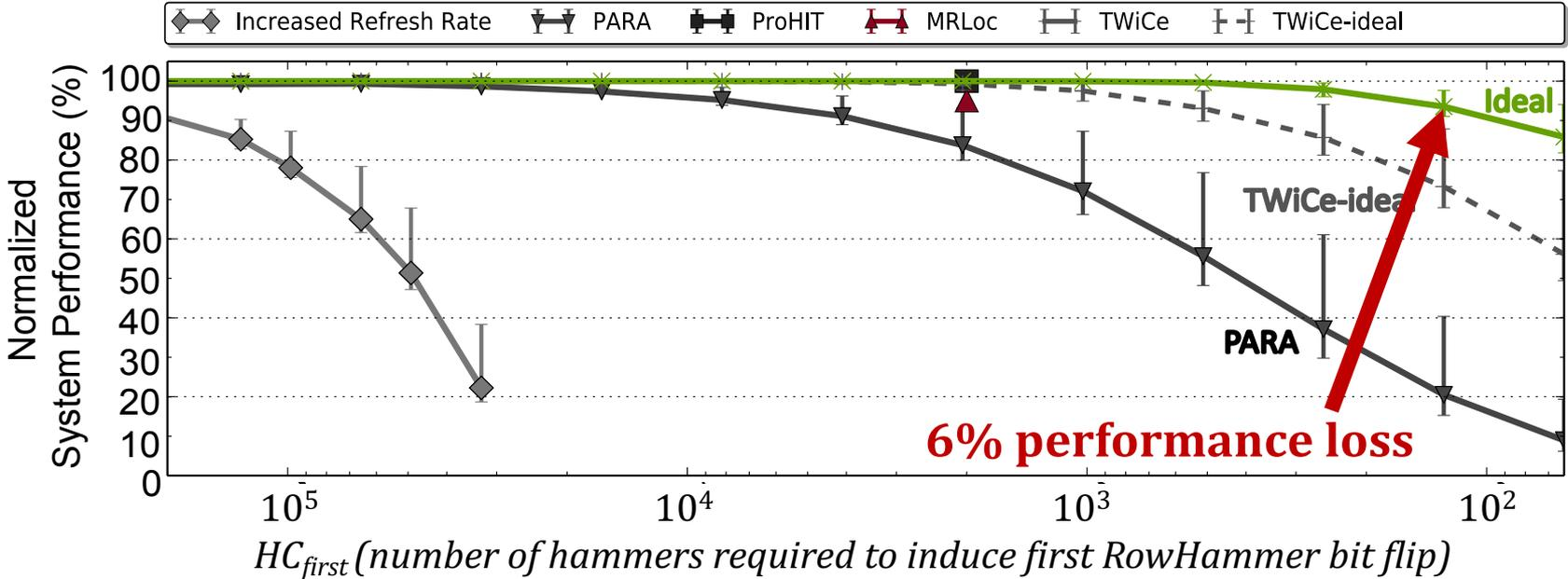
**Ideal mechanism** issues a refresh command to a row **only right before** the row can potentially experience a RowHammer bit flip
