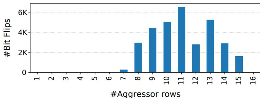
**Fig. 11: Bit flips vs. number of aggressor rows.** Module  $A_{15}$ : Number of bit flips in bank 0 as we vary the number of aggressor rows. Using SoftMC, we refresh DRAM with standard  $\tau_{REFI}$  and run the tests until each aggressor rows is hammered 500K times.
