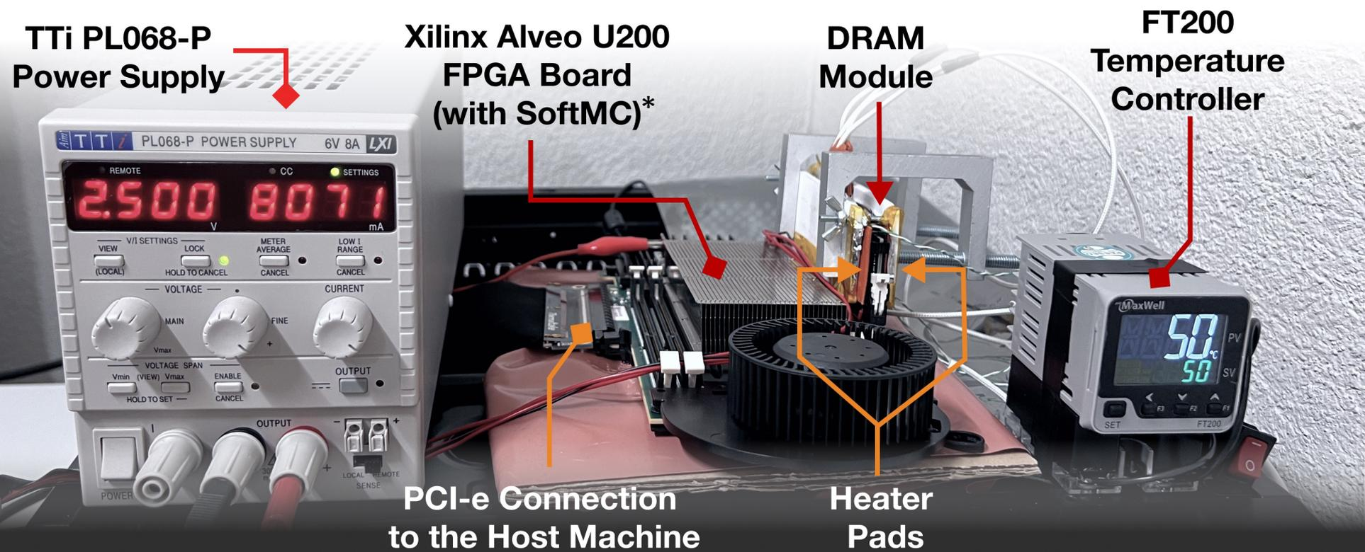
Fine-grained control over DRAM commands, timing parameters ( $\pm 1.5\text{ns}$ ), temperature ( $\pm 0.1^\circ\text{C}$ ), and wordline voltage ( $\pm 1\text{mV}$ )
