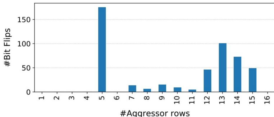
**Fig. 10: Bit flips vs. number of aggressor rows.** Module  $C_{12}$ : Number of bit flips in bank 0 as we vary the number of aggressor rows. Using SoftMC, we refresh DRAM with standard  $\tau_{REFI}$  and run the tests until each aggressor rows is hammered 500K times.
