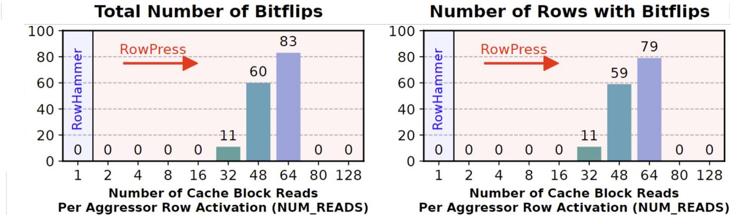
**Key Idea:** A proof-of-concept RowPress program keeps a DRAM row open for a longer period by **keeping on accessing different cache blocks in the row**
