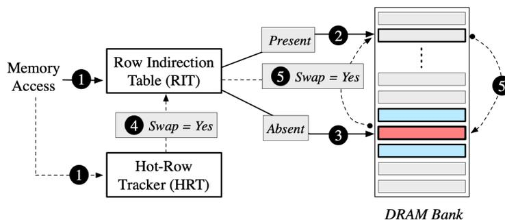
**Figure 2: Overview of the Randomized Row Swap (RRS).** The Row Indirection Table (RIT) is checked to determine if the access should go to original or remapped location. The Hot-Row Tracker (HRT) identifies rows that must undergo swap.
