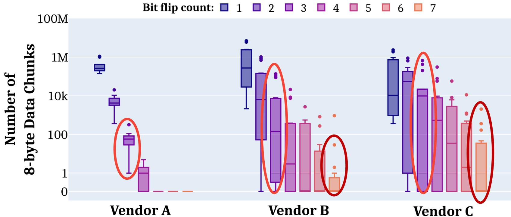
Modules from all three vendors have many **8-byte data chunks** with **3 and more (up to 7) RowHammer bit flips**
