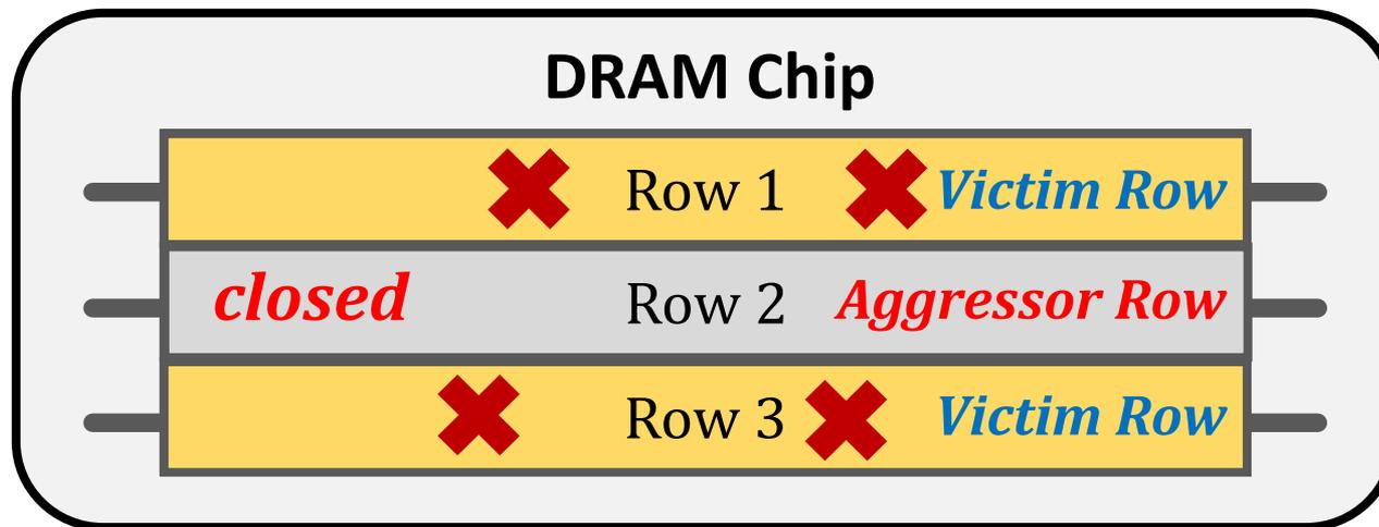
Repeatedly **opening (activating)** and **closing** a DRAM row **many times** causes **RowHammer bitflips** in adjacent rows
