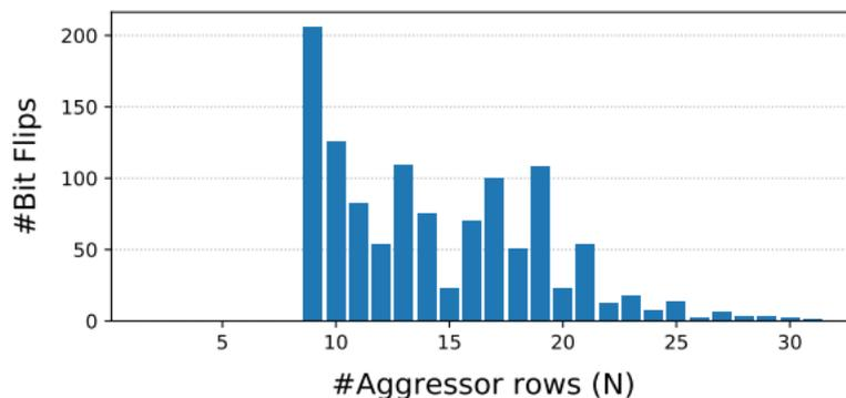
**Fig. 13: Bit flips vs. number of aggressor rows.** Module  $A_{10}$ : Number of bit flips triggered with  $N$ -sided RowHammer for varying number of  $N$  on Intel Core i7-7700K. Each aggressor row is one row away from the closest aggressor row (i.e., VAVAVA... configuration) and aggressor rows are hammered in a round-robin fashion.
