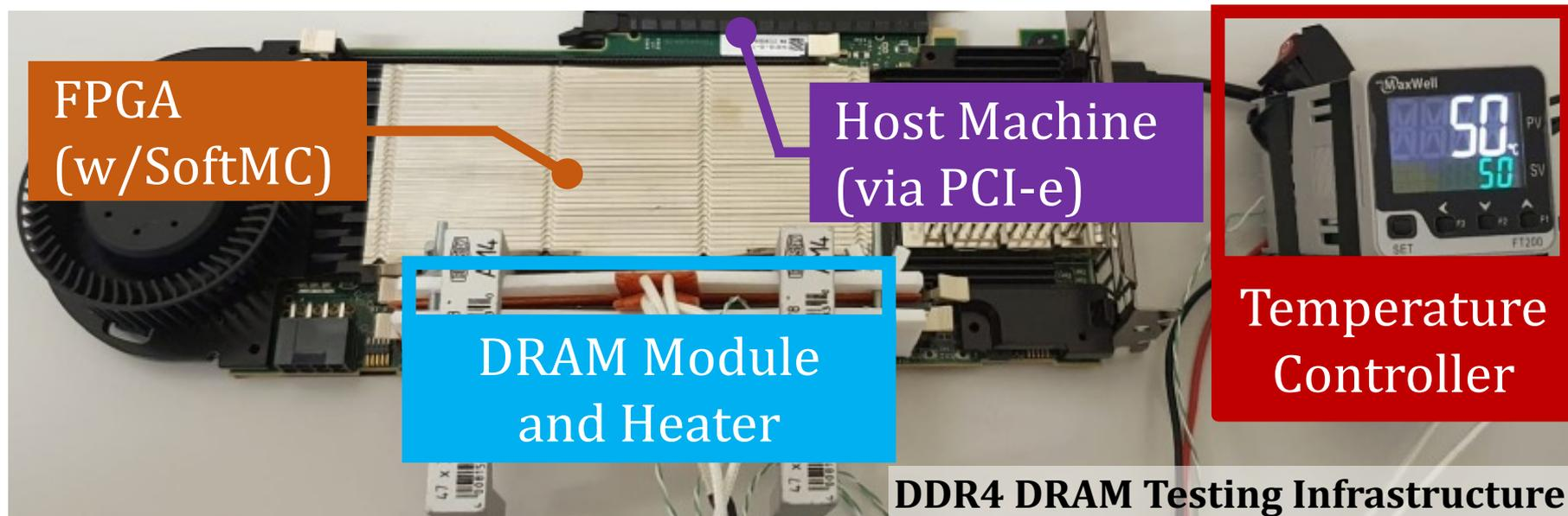
Fine-grained control over **DRAM commands**, **timing parameters** and **temperature ( $\pm 0.1^{\circ}\text{C}$ )**
