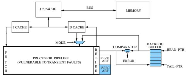
Figure 3. Microarchitecture support for MBI.
