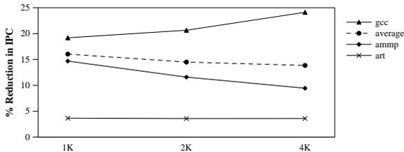
Figure 5. Sensitivity of the IPC overhead to the size of the backlog buffer. Y-axis represents the IPC overhead and X-axis represents the number of entries in the backlog buffer.
