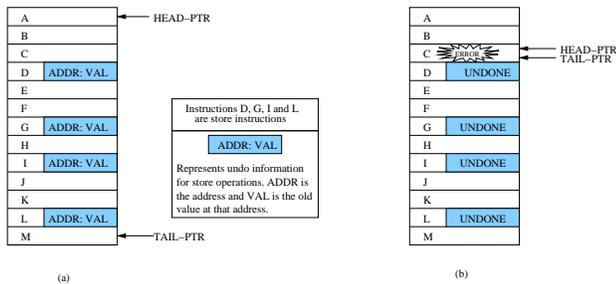
Figure 7. (a) Extending the backlog buffer to keep track of undo information for store instructions. (b) An example of error correction with the undo mechanism.
