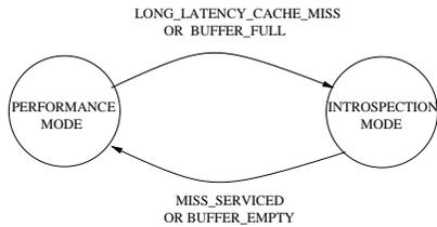
Figure 2. State machine for the MBI mechanism.
