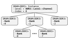
Figure 1. Tree of DDR3 state-machines
