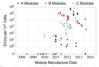
Figure 1. Normalized number of errors vs. manufacture date
