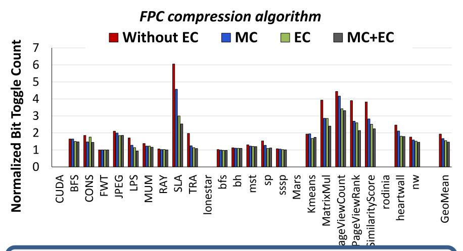
MC is effective in reducing the bit toggle count But less effective than EC
