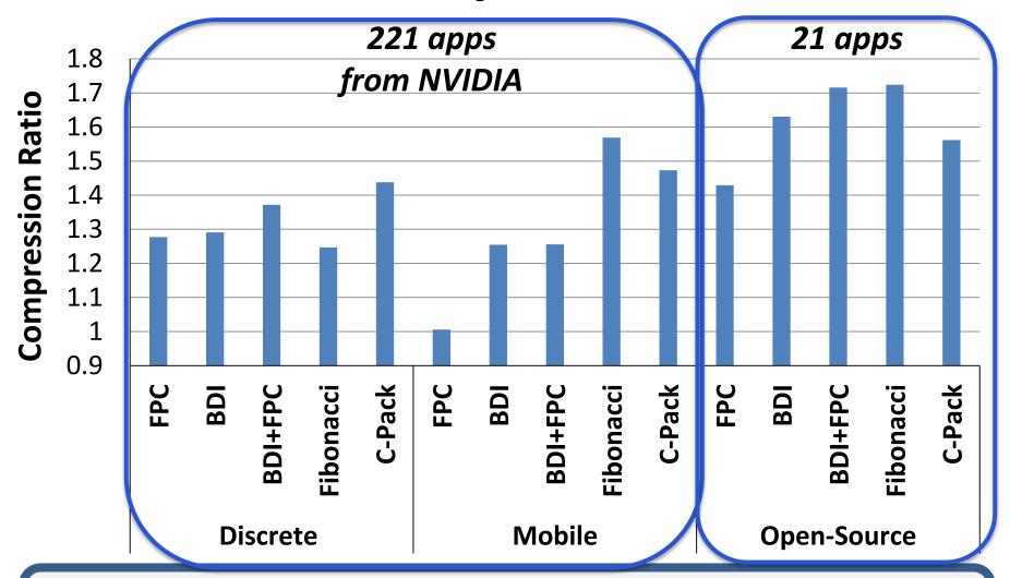
Compression is effective in providing higher bandwidth
