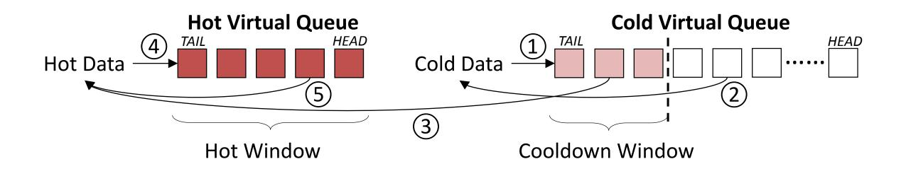
5. On a write hit in hot virtual queue, the data is pushed to the tail.
