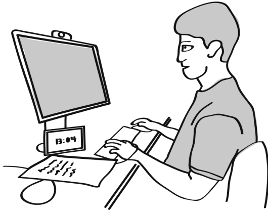
Figure 1. A sketch of the testing environment used in the study, showing the eye-tracking equipment (top of monitor), test instructions, the electrode cable extending from the participant’s left hand, and a digital clock for participants to keep track of time.
