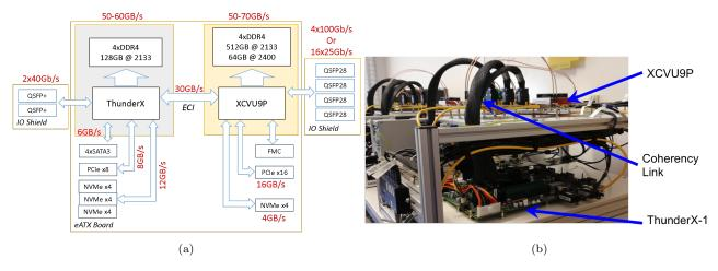
Figure 1: (a) Architectural schematic of Enzian and (b) photograph of the first operational prototypes
