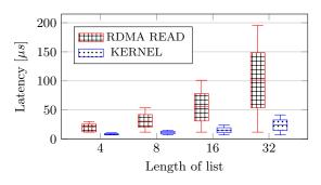
Figure 3: Traversing a remote linked list using conventional RDMA READ versus using the remote FPGA as memory controller implementing an RPC interface. Whiskers indicate the 1st and 99th percentile. Value size 64 B
